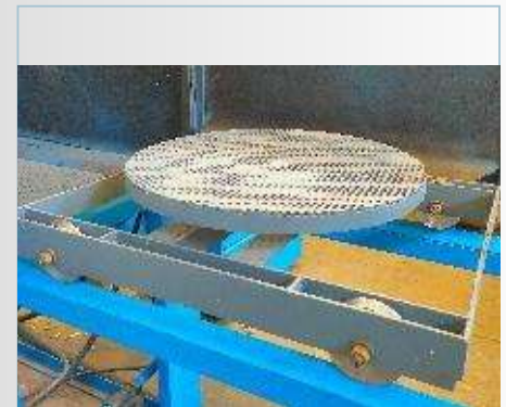
Work Car with Turn Table and Mounted Track Extension
